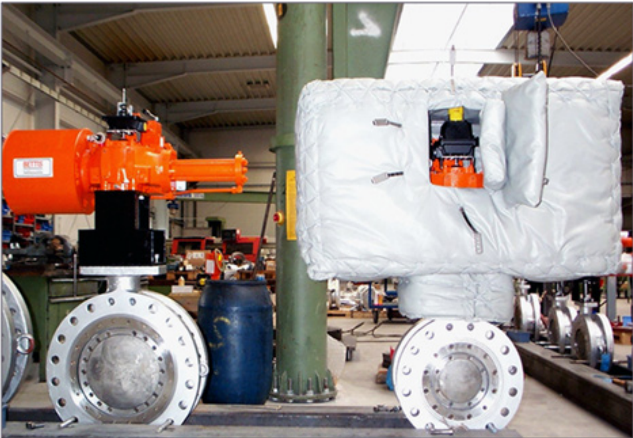
Figure 6.20.2.-1: Butterfly Type LTR 43 with Darmatt fire protection system
